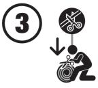
While keeping the mat firmly under downward pressure, carefully cut the retaining band(s).
